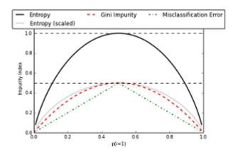
▶ Relation between impurity and the class probabilities. All impurity measures are maximized at  $p_1 = 1/2$  and minimized at  $p_1 = 0$  and  $p_1 = 1$ .
